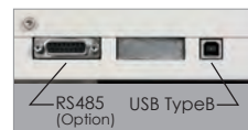
● A PC connector (USB Type B) is installed on the back of the unit RS485 (left side), USB TypeB (right side)
